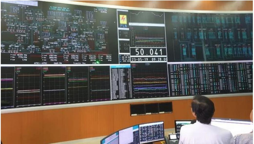
Gambar 1. 11. scada control centre
